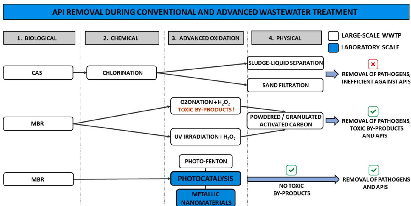
Fig. 1. Overview of conventional and advanced wastewater treatment techniques.
