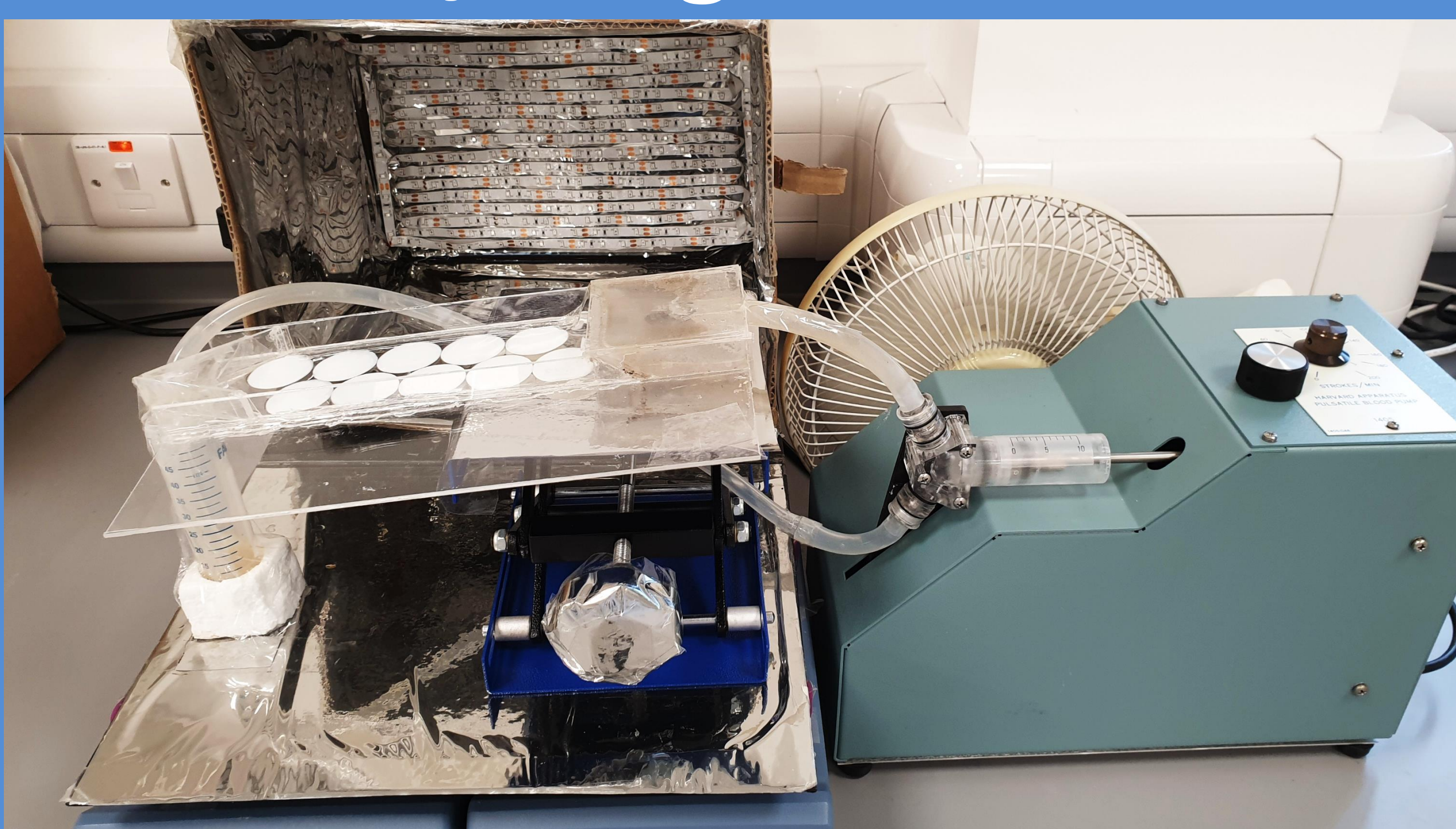
ZnO thin-film coated borosilicate slides in plate bed photoreactor
